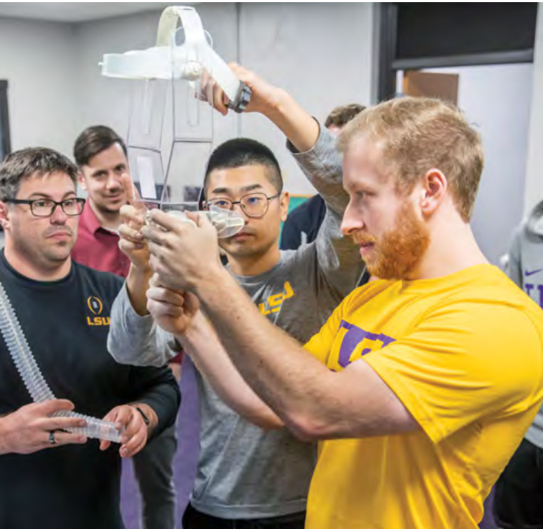
Pennington Biomedical researchers are using their equipment to test LSU athletes. The VO2 Max test measures the maximum amount of oxygen an athlete can use during intense exercise.
