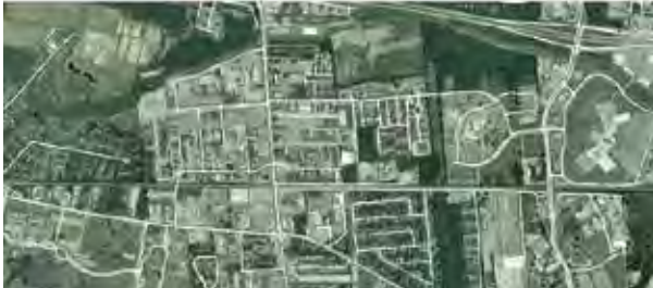
ABOVE —Mid City has an unbroken street grid, but urban areas built after World War II are not linked, causing traffic to be funneled to main roads, which become clogged.
