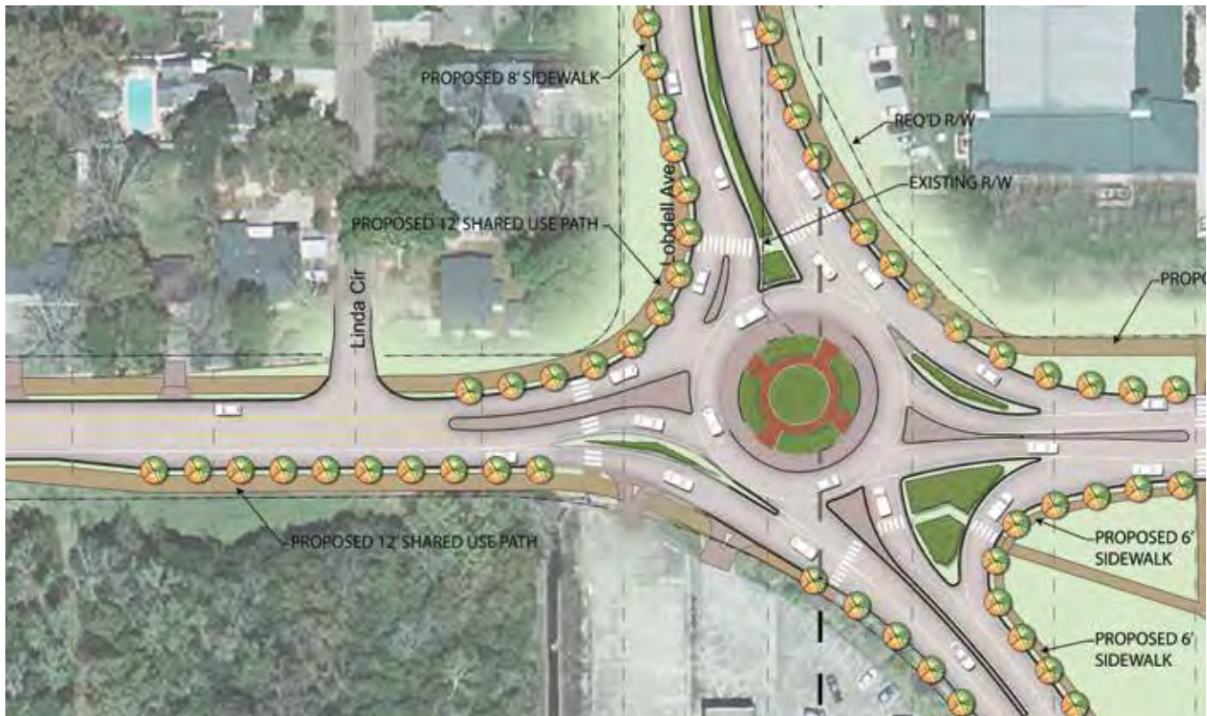
A state projects will reduce Government Street to three lanes – two lanes for driving, a center lane for turning – flanked by bike lanes, with medians along the way for safety. The “road diet” will reconfigure Government from I-110 to Independence Park, where a roundabout (above) will reduce wait times.
