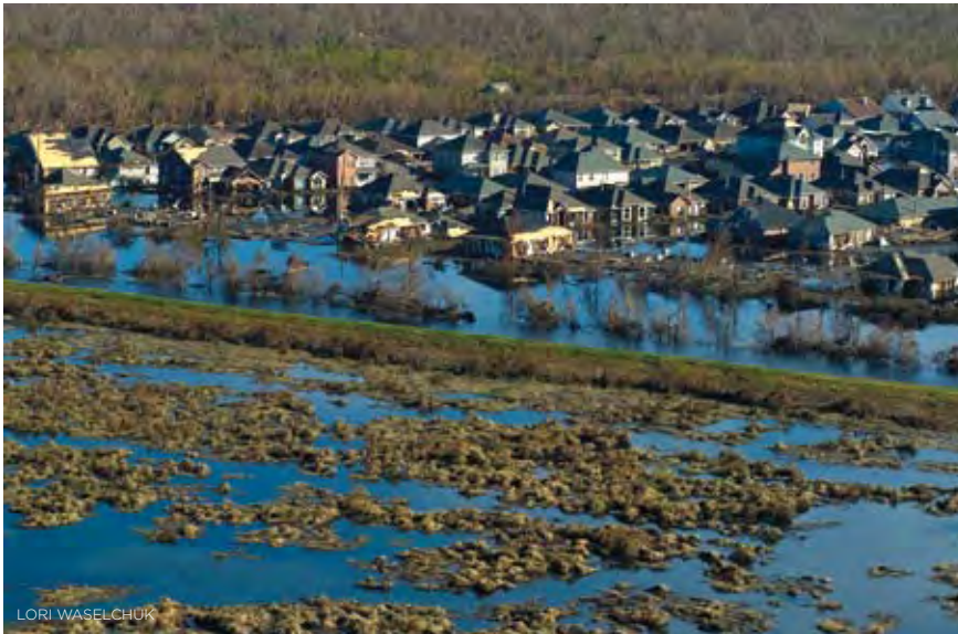
Marsh balls accumulated inside and outside the levee which was supposed to protect a neighborhood in St. Bernard Parish south of New Orleans.
