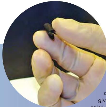
Rensselaer researchers created the battery by infusing paper with aligned carbon nanotubes, which gives the device its black color. The nanotubes act as electrodes and allow the storage devices to conduct electricity.
