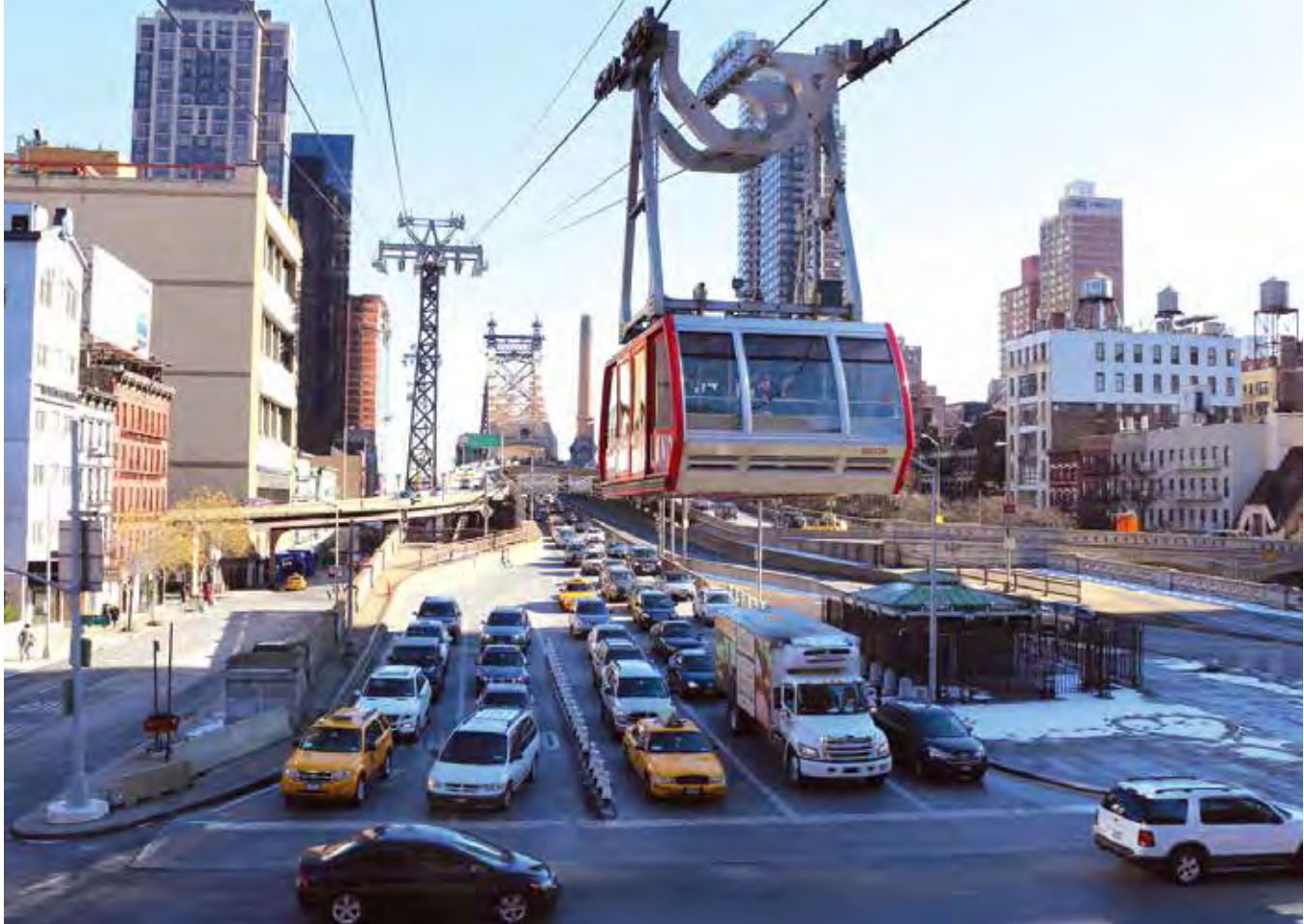
A tram connects Roosevelt Island to the Upper East Side of Manhattan over the East River in New York. Each of two cabins has a capacity of 110 people. The trip is three minutes.
